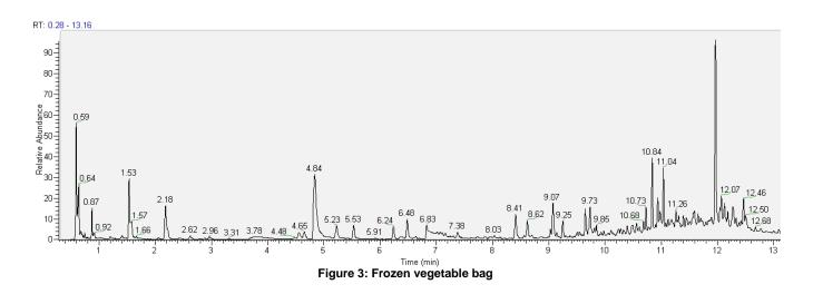
Notable for the frozen vegetable bag was the presence acetone at 1.53 minutes and methacrolein at 2.18 minutes. Methacrolein is an unsaturated aldehyde used in the manufacture of polymers or resins.
