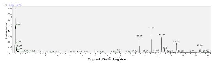
The late eluting peaks between 10-13 minutes for the boil in the bag rice packaging were deodecane, tridecane, tetradecane, pentadecane and hexadecane respectively.
