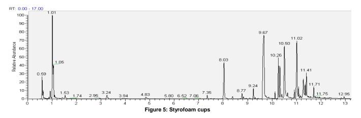
Styrene, as expected, eluted at the retention time of 9.24. Also notable is the presence of benzene at 3.24 and phenol is also present at 10.26
