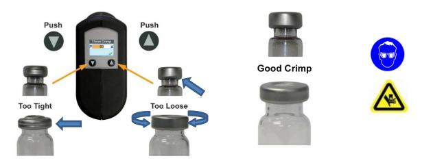
Check that the cap is neatly crimped all the way down to the bottom side of the vial neck.
