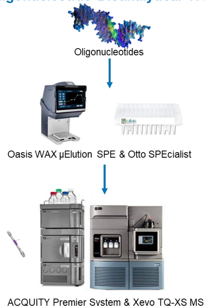
Figure 1. Standardized and semi-automated sample preparation and LC-MS/MS bioanalytical workflow using Oasis WAX SPE 96-well plate in the μElution format with the Otto SPEcialist positive pressure manifold to streamline the sample preparation process, maximize productivity, reduce errors, and improve analytical method performance.
