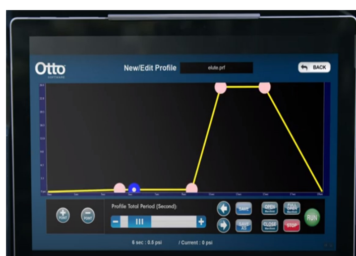
Figure 3. Visual representation of a pressure profile run on the Otto Software. The Otto SPEcialist will use a pressure profile to autonomously apply positive pressure to the SPE sorbent bed.
