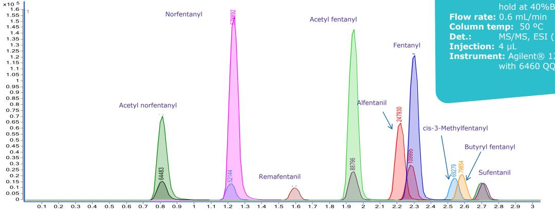
**Column:** Ascentis Express Biphenyl, 5 cm x 2.1 mm, 2.7 µm Mobile phase 0.1% formic acid in water **A: B:** 0.1% formic acid in methanol **Gradient:** 40%B to 50%B in 2 min, to 80%B in 1 min, hold 80%B for 1 min, to 40%B in 0.1 min and hold at 40%B for 1.4 min MS/MS, ESI (+), MRM Instrument: Agilent® 1290 Infinity II with 6460 QQQ
