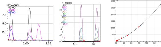
Figure 5: Butane and isobutane SIM signal at 10 µg in headspace, calibration peaks, and calibration curve.
