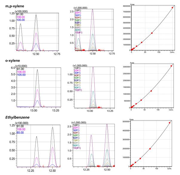
Figure 8: Xylene isomers and ethylbenzene SIM signal at 10 µg in headspace, calibration peaks, and calibration curve.
