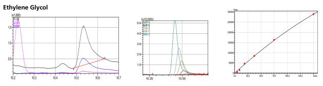
Figure 4: Ethylene glycol SIM signal at 4 µg in headspace, calibration peaks, and calibration curve.
