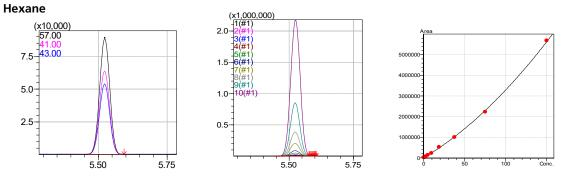
Figure 7: Hexane and isomers SIM signal at 10 µg in headspace, calibration peaks, and calibration curve.
