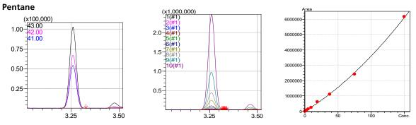
Figure 6: Pentane and isomers SIM signal at 300 ng in headspace, calibration peaks, and calibration curve.
