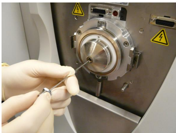
Figure 3: Installation of the SICRIT® Inlet capillary.
