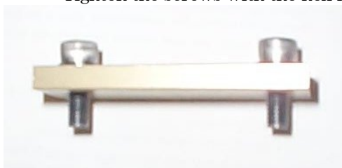
Figure 2. Metal plate with two M6 screws and spring washers attached
