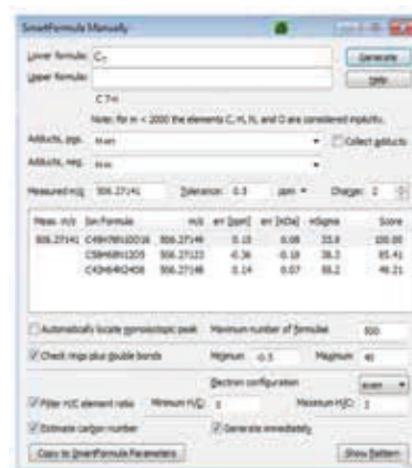
Figure 5: SmartFormula results for peak at m/z 507.27141. Three molecular formula hits were generated within a 0.5 ppm mass accuracy window
