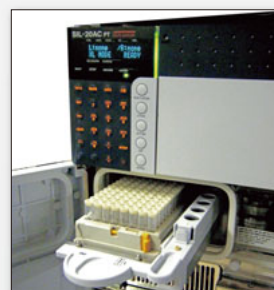
Automated derivatization reaction using an autosampler
