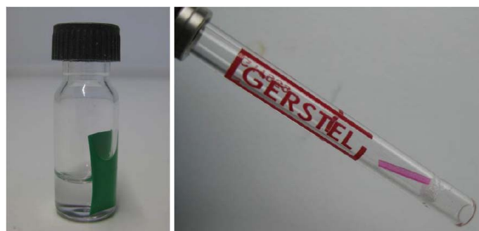
Figure 3. A sample extracted using method 1 (LE) inside a 1.5mL vial and a sample extracted using method 2 (TD) inside a TDU thermal desorption tube.
