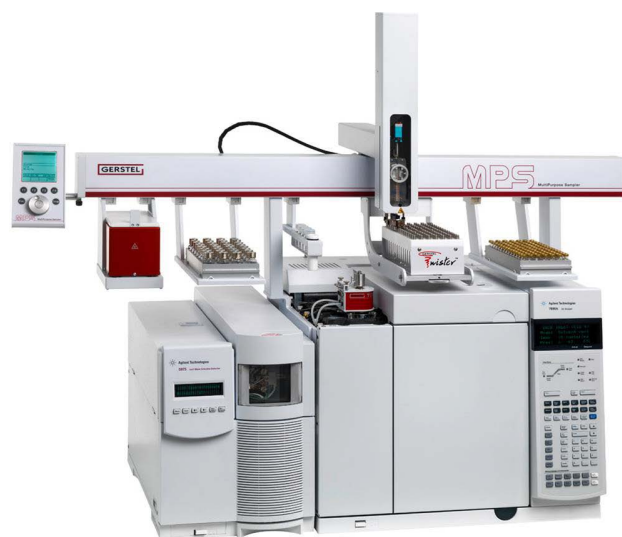
Figure 1. GC/MS system used for the determination of extractables from materials.
