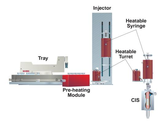
**Figure 1.** *Gerstel Multi Purpose Sampler in standby (left) and injection mode (right).*
